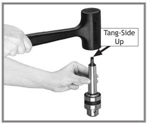
**Figure 18.** Seating the arbor into the chuck.
